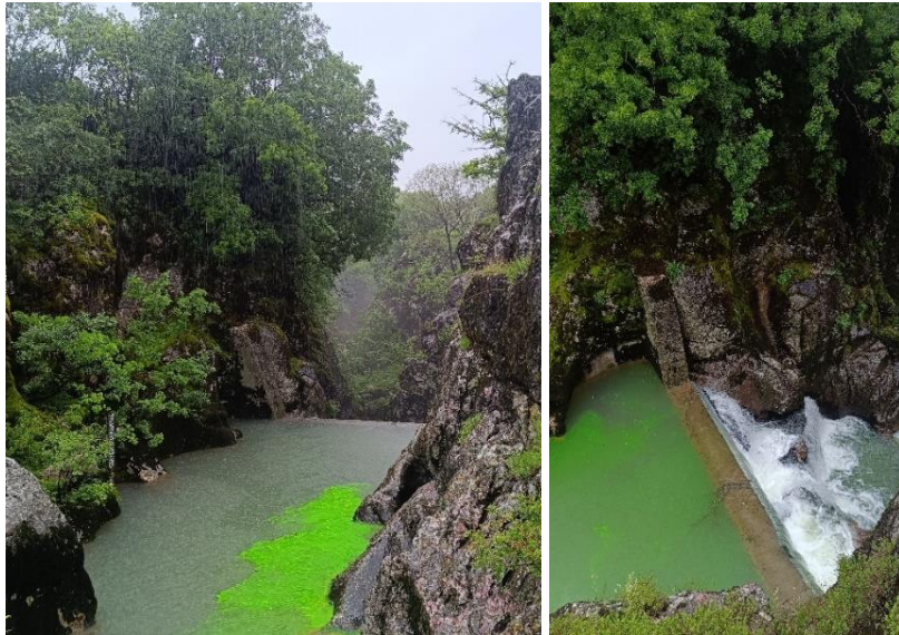
Performing of tracer test on the Ključka Reka river in Cernica Polje
